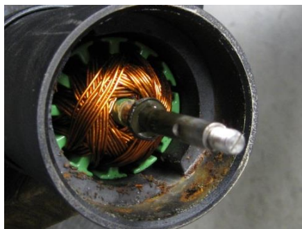
Figure 3 (Water damage to the lower unit)
