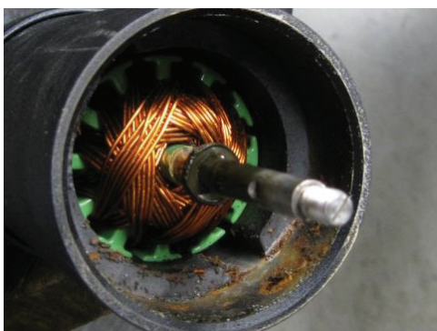
Water damage to the lower unit
